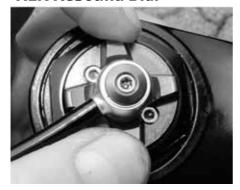
Rotate the red rebound dial in the "--" direction (counter-clockwise) to increase rebound speed (faster).
